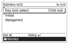
Select [Child lock] or [Part lock] with the [Cursor button (Up/Down)], and press the [Enter button].
