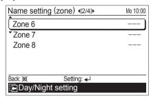
Select the zone to be named with the [Cursor button (Up/ Down)], and press the [Enter button].
