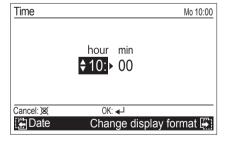
To complete the setting, press the [Enter button]. The screen returns to the "Date and Time" screen.
