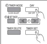
Press the DAY (DAY OFF) button and TIMER SET button simultaneously for 2 seconds or more to activate the child lock function and lock all of the buttons on the remote controller except the START/STOP button, SET TEMP. buttons, MODE button, and FAN button. Press the buttons again for 2 seconds or more to deactivate the child lock function.
