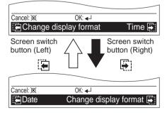
**NOTE:** These buttons are active only when any combinations of and the relevant screen names are displayed in the black field at the bottom of the screen.
