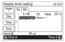
Select the room-temperature sensor with the [Cursor button (Up/Down)]. Then press the [Cursor button (Right)] to move the cursor to next setting item.
