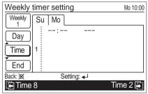
(2) Select the pattern number with the [Cursor button (Up/ Down)]. Then press the [Cursor button (Right)] to set the time setting of On/Off timer, On/Off, operating mode, and temperature for the current selected pattern.
