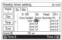
After you select all the applicable zones, press the [Enter button] to complete the individual setting of zone control.
