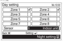
Each time you press the [Cursor button (Up/Down)], displayed sensor switches as follows.
