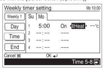
(6) When you selected [On] (On timer), adjust the value to the desired temperature with the [Cursor button (Up/ Down)].
