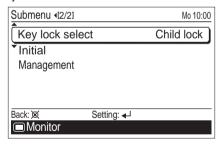
2 Select [Child lock] or [Part lock] with the [Cursor button (Up/Down)], and press the [Enter button].
