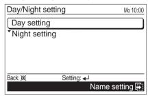
Select [Day setting] for the registration of group "Day", and select [Night setting] for the registration of group "Night", with the [Cursor button (Up/Down)]. When you press the [Enter button], registerable zones and roomtemperature sensor are displayed.
