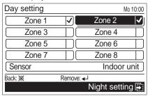
To remove the check mark, adjust the cursor to the zone name to be unchecked, and press the [Enter button] again.
