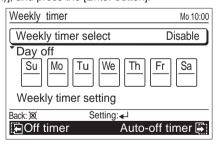
Select any of [Weekly 1], [Weekly 2], or [Disable] with the [Cursor button (Up/Down)], and press the [Enter button].
