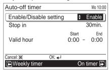
For [Stop in], adjust the timer with the [Cursor button (Up/Down)]. To complete the setting, press the [Enter button].
