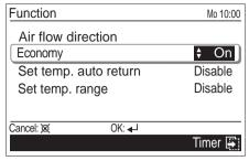
When you return to the "Monitor" screen, the icon is displayed. To check the function, press the [Enter button] and select the icon with the [Cursor button (Left/Right)].
