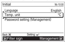
Select [°C] or [°F] with the [Cursor button (Up/Down)] and press the [Enter button].
