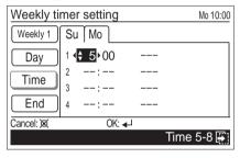
(4) Select [On] (On timer) or [Off] (Off timer) with the [Cursor button (Up/Down)]. When you selected [Off] (Off timer) here, skip following step (5) and (6).
