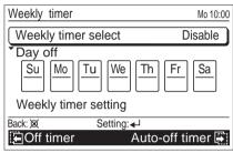
To change the setting, select the item with the [Cursor button (Up/Down)], and press the [Enter button].
