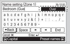
4 Set the cursor to [End] with the [Cursor button], and press the [Enter button] to finalize the name registration.
