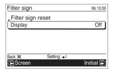
Select [On] or [Off] with the [Cursor button (Up/Down)], and press the [Enter button].
