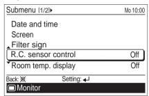
2 Select [On] or [Off] with the [Cursor button (Up/Down)], and press the [Enter button].
