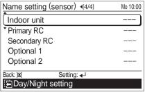
If any names have been registered for the sensors already, the registered names are displayed instead of "---" on this screen.
