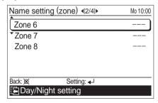
Select the zone to be named with the [Cursor button (Up/ Down)], and press the [Enter button].
