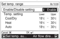
For [Temp. setting], select mode with the [Cursor button (Up/Down)] and press the [Enter button].
