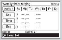
Press the [Enter button]. Then select [Weekly 1] or [Weekly 2] with the [Cursor button (Up/Down)], and press the [Enter button].
