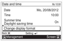
"Change display format" screen is displayed. Select the setting items (Date format or Time format) with the [Cursor button (Left/Right)] and set with the [Cursor button (Up/Down)].
