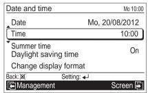
2 "Time" screen is displayed. Select the setting items (hour, min., or AM/PM) with the [Cursor button (Left/Right)] and set with the [Cursor button (Up/Down)]. When setting the minutes, setting can be completed quickly if the button is pressed continuously.
