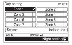
Select zone to be registered in the group with the [Cursor button]. When you press the [Enter button], a check mark is displayed.
