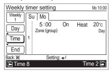
(8) When setting the other days of the week continually, perform procedures in step 4 and 5. To finalize the setting you have set in step 5, select [End] with the [Cursor button (Up/Down)], and press the [Enter button].
