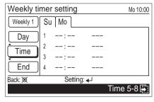
(2) Move the cursor between each pattern number with the [Cursor button (Up/Down)], and press the [Cursor button (Left/Right)] to set the time setting of On/Off timer, On/ Off, operating mode and temperature for each pattern.
