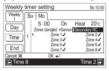
Select applicable zone name with the [Cursor button (Left/Right)], and press the [Cursor button (Up/Down)] to mark a check.
