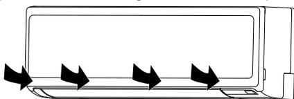
**NOTE:** If dirt accumulates on the air filter, airflow will be reduced, operating efficiency will lower, and the noise will increase.
