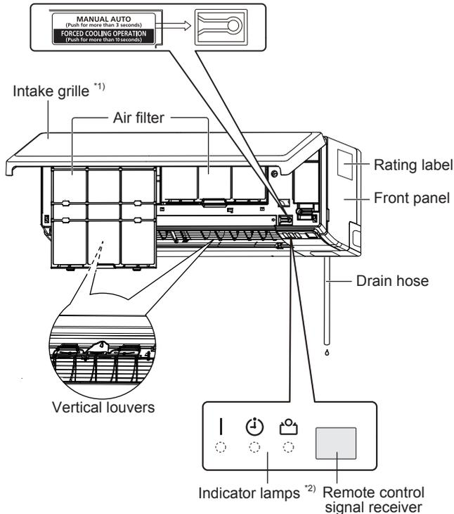
\*1) Before starting operation, make sure that the intake grille is closed completely. Incomplete closing may affect the proper function or performance of the product.
