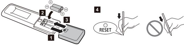
1~3. Put batteries as shown in the figure above.
