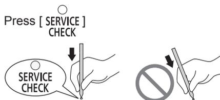
The remote controller enters to the Service check mode and “” will appear on the remote controller display.
