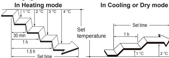
After the set time has elapsed, the air conditioner operation turns off.
