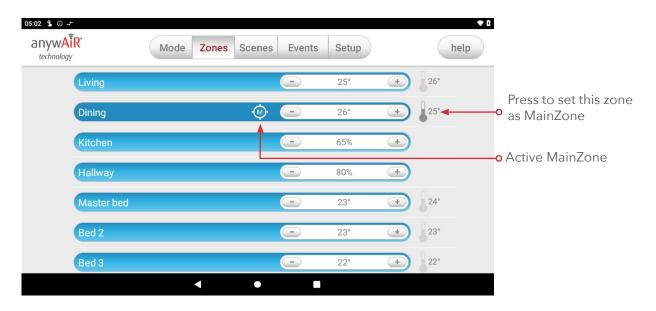
This feature can be particularly important when you have an unusually high requirement for air conditioning in a particular area. For example, a group of people watching a movie in Theatre room with all the electronic A/V equipment turned on will have a larger requirement for air conditioning than in other rooms in the house. Setting the Theatre as MainZone will ensure that the system continues running until the temperature set-point for that room is achieved.
