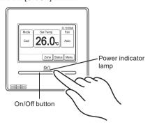
The Power indicator lamp remains lit while the indoor unit is operating.
