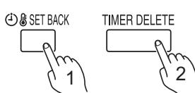
Press the SET BACK button, and then press the TIMER DELETE button while the Set back confirmation display is displayed. Even if the SET BACK button is pressed again, the Set back timer will be cancelled.
